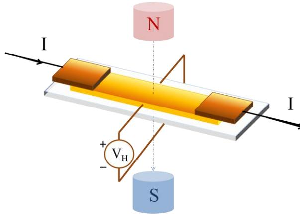
**Fig. 1:** Hall Voltage ( $V_H$ ) developed across a current-carrying conductor in a magnetic field
